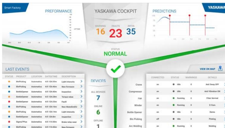
With the YASKAWA Cockpit Yaskawa is developing a new central software platform for networked production environments. (Source: Yaskawa)
