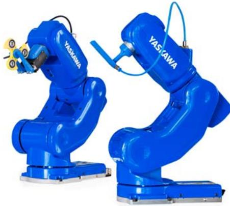
Yaskawa has extended the Motoman robot portfolio to include its smallest model: with a range of 350 mm the new MotoMINI has a lifting capacity of 500 g. (Source: Yaskawa)
